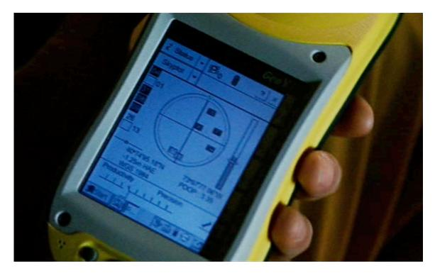
Numbers for latitude and longitude are visible along with a negative value for height above the ellipsoid, a value for positional dilution of precision and that the unit is set to WGS 1984 as the coordinate system. The Skyplot shows four satellites, but the number next to the satellite icon at the top appears to show zero. My version of TerraSync is different from the version on this unit so I am unable to correlate some of the buttons shown next to the Start button at the base of the screen.
